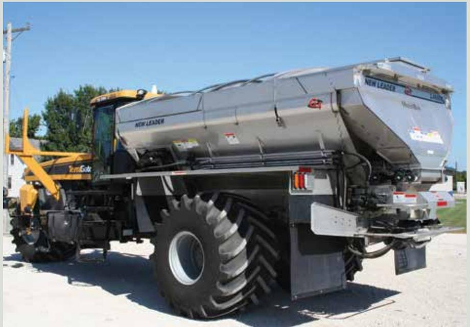
*Gold-Eagle has purchased a New Leader L 4000G4 spreader with four boxes for dry fertilizer. This spreader can be used for single or variable-rate application to broadcast phosphorus, potassium, sulfur, and zinc from the four bins, either independently or together. The boxes have the capacity to hold approximately 5 tons each of potassium and phosphorus, and 2/3 ton of sulfur and zinc. All bins are made of stainless steel to prevent corrosion. We'll put the New Leader into service this fall.*
